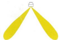
Double Symmetric 25° beam angle
